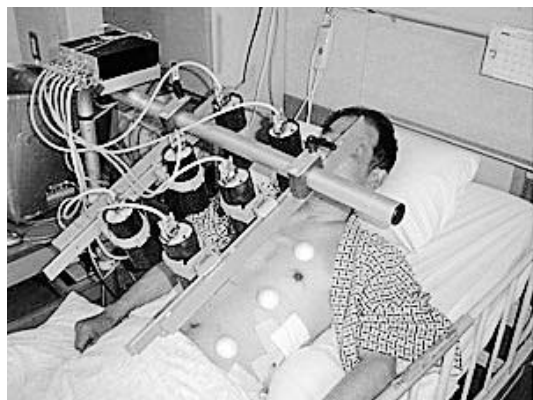
図1 RMMIを用いた胸壁運動測定 (RMMI; Respiratory Movement Measuring Instrument)
